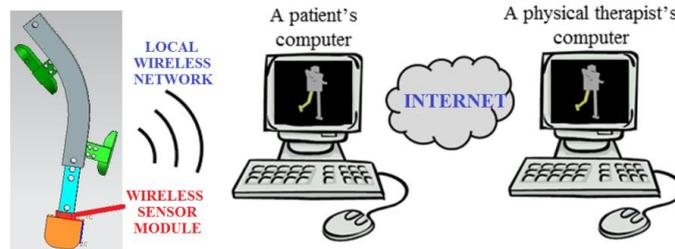
Fig. 3 Biofeedback system in crutch
